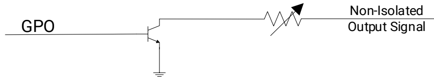
Figure 5-3 Internal Circuit of Output Signal
